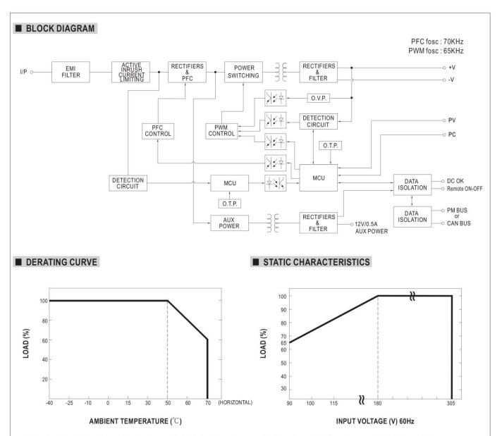
※ For 100V model charging mode, output current is 20% rated min. when operating tempature at -40°C, and can reach 100% above -30°C.
