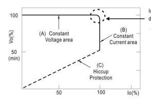
Typical LED power supply I-V curve
